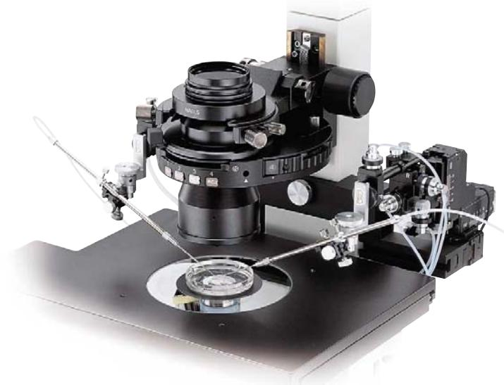
The IX2-MLWCD comes equipped with optical component RC1 (for 10X objective), RC2 (for 20X objective), RC3 (for 40X objective) and a polarizer to adjust the contrast.
